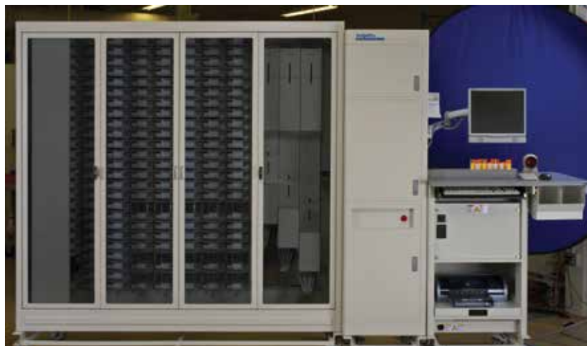
Then: The SP 200/OCC, above, the company's original robot (robotic prescription dispensing system).
